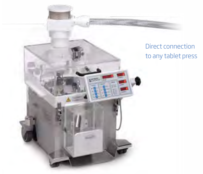
The dust-proof version of the UTS 4.1-S20 with single tablet feeder guarantees safety at work
