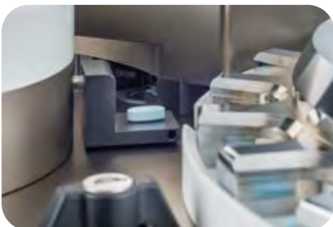
Precise tablet positioning (patented stamp)
