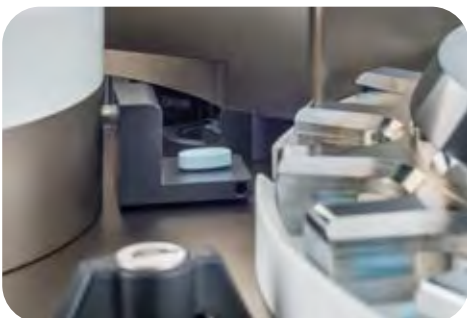
Precise tablet positioning (patented stamp)
