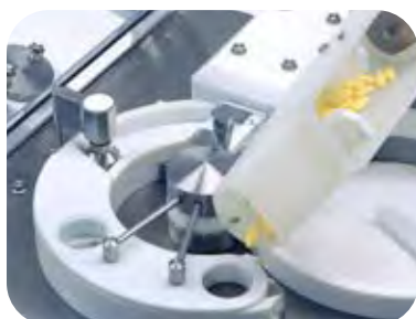
Patented radial transport rake
